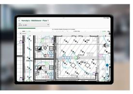
The Visual Installer mobile app streamlines lighting control installation and as-built workflows. Using project floor plans and risers that are made available in the app, users scan lighting control devices to capture real-time installation status, exact device locations, and design changes. In addition, the
