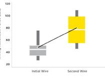
Instead of loosening, EdgeConnect terminations hold wires tighter when subjected to vibration and temperature cycling.
